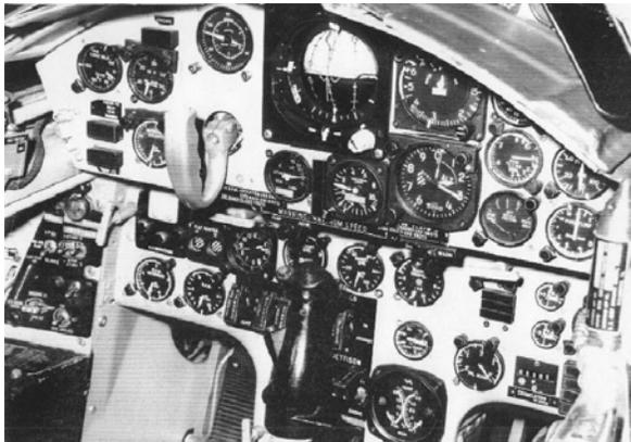
Figure 5. NF-104A Instrument Panel
